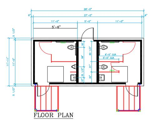
NOTE: LANDINGS, WALKWAYS, AND OR RAMPS ARE TO BE FIELD INSTALLED BY OTHERS AS REQUIRED TO MEET LOCAL HANDICAP REQUIREMENTS.
