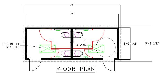
NOTE: LANDINGS, WALKWAYS, AND OR RAMPS ARE TO BE FIELD INSTALLED BY OTHERS AS REQUIRED TO MEET LOCAL HANDICAP REQUIREMENTS.
